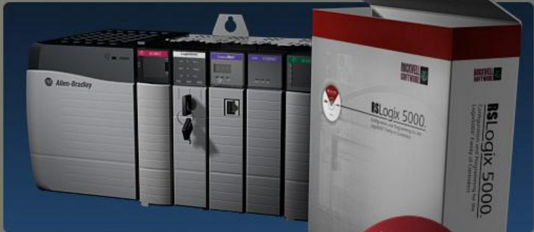
The ControlLogix system uses the RSLogix 5000 programming environment, can connect to the NetLinx open networks architecture, and offers a wide range of digital, analog, and specialty I/O modules.
